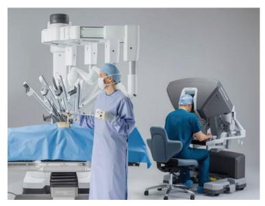
The robotic system employs a 3D camera, which yields high-definition depth perception of the surgical field at 10x power magnification, along with extremely precise surgical instruments. State-of-the-art controls can allow better dexterity than the human hand alone.
